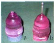
图1 热处理前(a)、后(b) 合成掺Ti蓝宝石晶体 Fig.1 Synthetic Ti-doped sapphire samples before(a) and after(b) heat treatment
