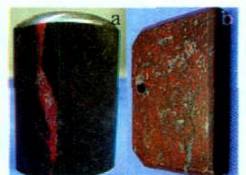
图2 含辰砂的钙质粉砂岩(a)和石英岩(b) Fig.2 Calc-siltstone(a) and quartzite(b) with cinnabar
